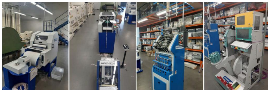
Figure 9: Spinning line from Mesdan: carding, drawing and roving, spinning, and winding (from left to right)
